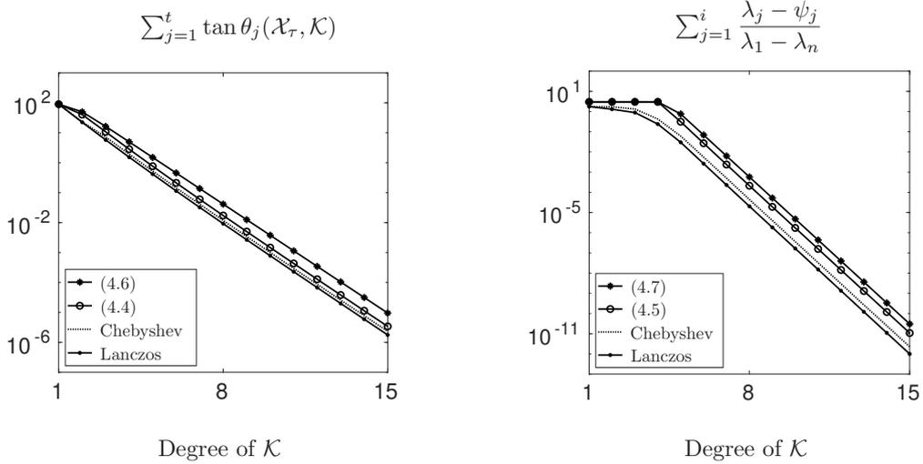
FIGURE 1. Numerical comparison of the new bounds (4.4) and (4.5) with the relevant bounds (4.6) and (4.7) based on [15] accompanying the block Chebyshev and Lanczos methods; see Example 1 with  $p = 3$ ,  $\tau = \{1, 2, 3\}$ ,  $t = 3$  and  $i = 3$ .
