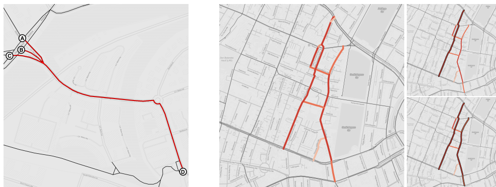
FIGURE 6 Example of gap clusters, and of the declustering heuristic. Left: Shown in red, on C.F. Richs Vej. The three gaps AD, BD and CD overlap and have similar closure benefits B(\mathbf{g}) . Therefore, the three gaps are merged into one gap cluster to be handled jointly. Right: A declustering heuristic can help deciding which parts to retain and which ones to discard. The links of the shown gap cluster are colored by betweenness centrality; darker tones represent higher values. The black borders indicate the declustered gaps after one and two runs of the heuristic.
