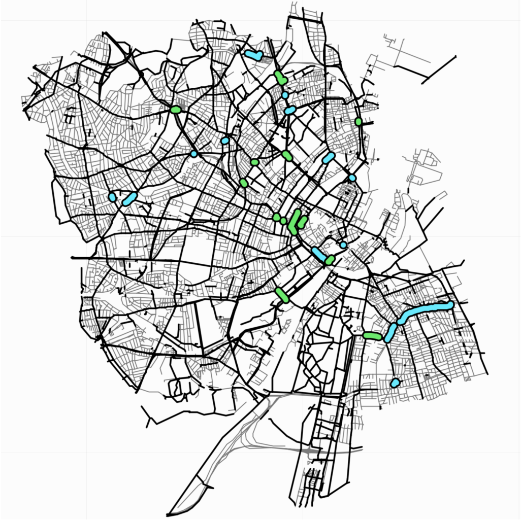
FIGURE 12 Errors in the list of top ranked gaps in Copenhagen. 29 out of 134 gaps identified by the IPDC procedure in the Copenhagen network that have been discarded as errors: data issues in light blue; parallel paths in light green.
