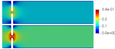
FIGURE 5. Reduced velocity \mathbf{u}_{f,N} at time-step t = 0.04s (top) and at time-step t = 0.05s (bottom). The velocity has been obtained with N_z = 15 reduced basis.
