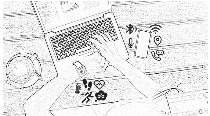
Fig. 1. Wearables and smartphones are two common passive sensing technologies, offering physiological data such as heart rate, skin temperature, physical activity and sleep and contextual data such as location, proximity and phone usage.
