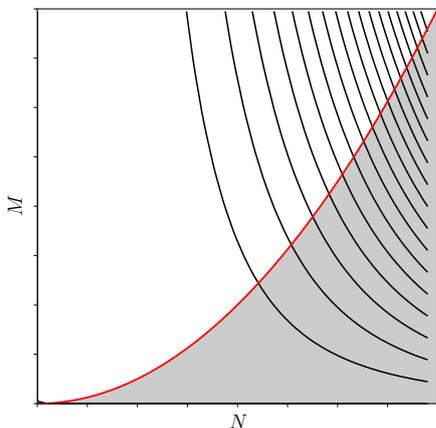
**Fig. 4.** Comparison between the efficiency of the meshfree and grid-based methods. The horizontal axis shows the grid resolution, while the vertical axis shows the number of coefficients per model parameter. The gray shaded area below the red curve  $M = N^2$  shows the models more efficiently inverted using the meshfree method. The black curves connect models with identical required CPU time per iteration of a grid-based model. See the main text for further details.
