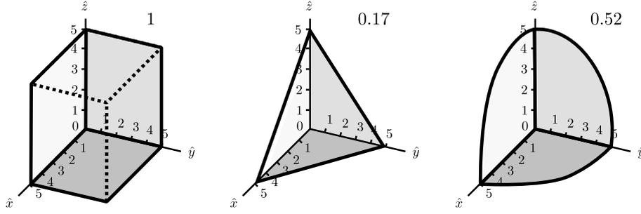
**Fig. A.1.** Schematic representation of three bases of the same order  $p = 5$  for approximating the spatial variation of the problem variables in the computational domain. The numbers in the top right part of each diagram indicate the fraction of the number of the considered basis functions with respect to the full basis in the left diagram.
