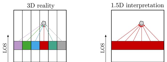
**Fig. 1.** Spatial coupling between lines of sight in a 3D (left) and in a 1.5D (right) model atmosphere. In 3D, the radiation field at a given point results from radiation transfer from different regions of the domain, both in the vertical and in the horizontal directions. In 1.5D, the horizontal variation is neglected. The 1.5D model can be sufficiently accurate in some cases but, in general, it often leads to serious errors in calculation of the line scattering polarization.
