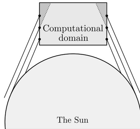
**Fig. 5.** Geometry of the illumination of the computational domain by the underlying solar surface using an angular quadrature. If the angular quadrature is identical at every point (see the inclined lines), artificial sharp jumps in the illumination at the boundary, which do not actually exist, will appear in the model. Such artifacts could make a full 3D inversion nearly impossible. The solution to this problem is to use a randomized quadrature at every pilot point.
