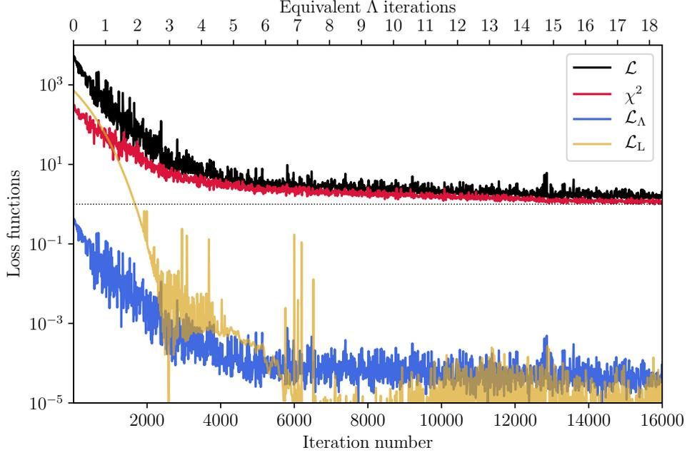
**Fig. 10.** Convergence of the stochastic meshfree method. The individual curves correspond to the respective terms in Eq. (27) shown in the legend. The bottom horizontal axis shows the number of stochastic iterations, while the top horizontal axis shows the CPU time in units of full  $\Lambda$ -iterations in a  $N^3 = 64^3$  grid-based model.
