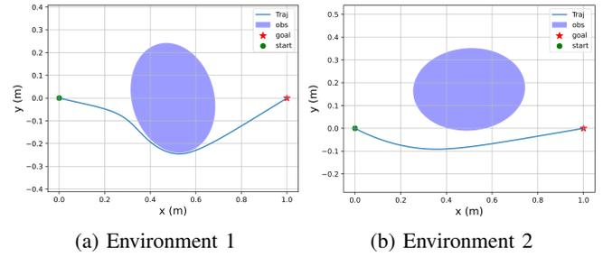
Fig. 1: Motivating example for safety-critical control for generalization to novel environments using a 2D double integrator. A hand-tuned  $K_\alpha$  for Environment 1 in (a) is used in the novel Environment 2 in (b). As can be seen, this results in a trajectory with a larger deviation from the obstacle in Environment 2. Thus, a well-tuned  $K_\alpha$  for one environment does not necessarily generalize to a different environment.
