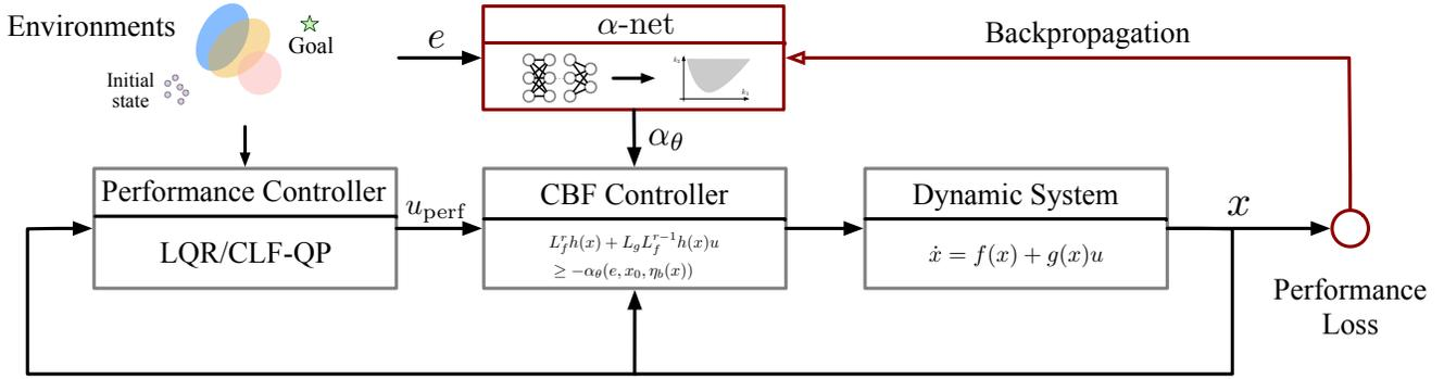
Fig. 2: The overall framework of the proposed approach, which includes two main components: a performance controller and a differentiable CBF-QP. The novel environment information,  $e$ , is an input to the performance controller and  $\alpha$  net. The performance loss computed along a trajectory will be backpropagated through the  $\alpha$  net, then the  $\alpha$  net outputs the parameters to construct the class  $\mathcal{K}$  function.
