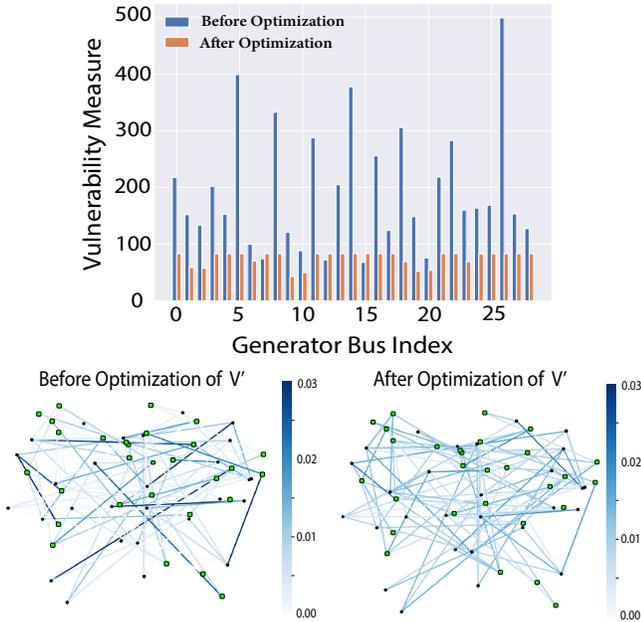
Fig. 4. In the bar plot,  $\hat{\mathcal{M}}_k(b_0)$  for each of the twenty-nine nodes corresponding to generator buses,  $k$ , is plotted in blue, and  $\hat{\mathcal{M}}_k(b^*)$  for each of the twenty-nine nodes corresponding to generator buses is plotted in orange. Below the bar plot, once again, the 57 bus-case system is plotted twice. In the left graph, edge weights correspond to original susceptance values,  $b_0$ , and in the right graph edge weights correspond to  $b^*$ .
