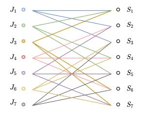
Fig. 7. Bipartite graph associated with the incident structure of a (7,3,1)-BIBD. Every pair of two jobs (colors) appear on exactly one server.
