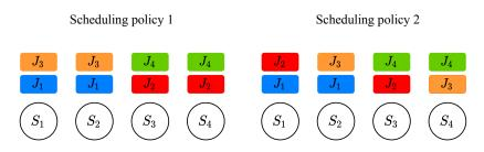
Fig. 2. Scheduling with overlapping queues. Despite introducing redundancy, scheduling policy 1 provides no diversity on the jobs' queuing time. Scheduling policy 2, on the other hand, provides diversity. A scheduling policy's ability to provide diversity can be measured by studying the resulting overlaps between the replicas of jobs.
