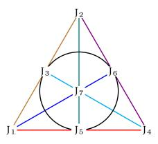
Fig. 5. (7,3,1)-BIBD where the seven points correspond to seven jobs. Each job is assigned to three servers (lines in the figure). Two different jobs (points) share only a single server (line).
