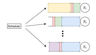
Fig. 1. Scheduling model: Jobs get redundantly assigned to servers. The scheduling is nonadaptive, i.e., it has no information about the workload in the queues. Observe that copies of two different jobs may be assigned to the same server. These overlaps are unavoidable and depend on the scheduling policy.
