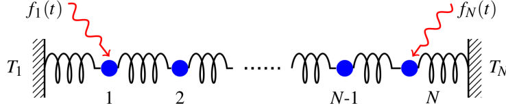
FIG. 1. Schematic representation of a chain of oscillators connected to two nonequilibrium reservoirs which exert active forces f_{1,N}(t) on the boundary oscillators.
