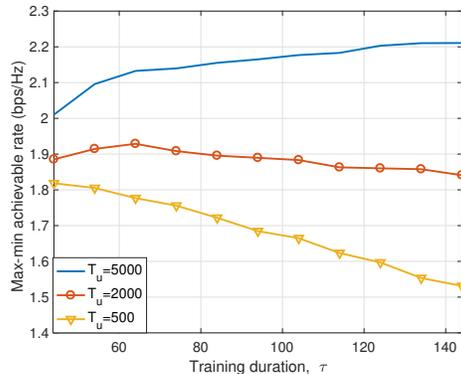
Fig. 5. Max-min achievable rate versus training duration,  $\tau$  under different length of fading block,  $T_u$ .
