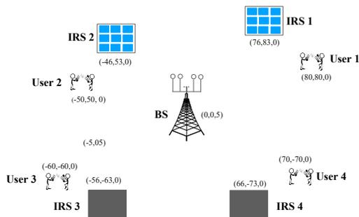
Fig. 8. Simulation setup for user-side IRSs.
