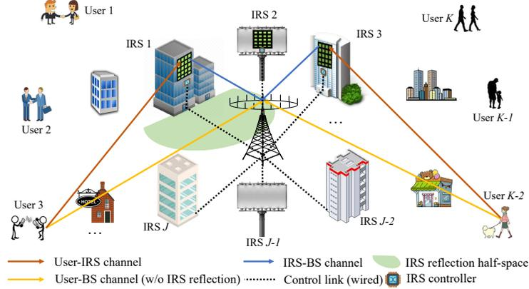
Fig. 1. A new architecture of BS empowered by multiple co-site IRSs in its vicinity.
