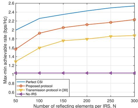
Fig. 6. Max-min achievable rate versus fading block length, Fig. 7. Max-min achievable rate versus number of reflecting elements per IRS,  $N$ .
