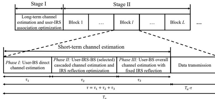
Fig. 2. Frame structure of the proposed transmission protocol.
