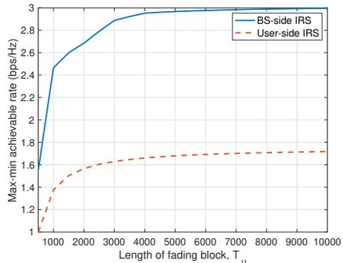
Fig. 9. Performance comparison between BS-side IRSs and user-side IRSs.
