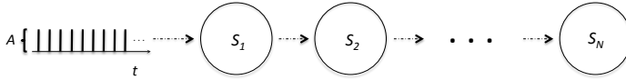
Fig. 1 Network diagram. A periodic train of Dirac stimuli is injected into S_1 ; for j \geq 2 unidirectional coupling provides communication between S_{j-1} and S_j via an instantaneous kick to the recovery variable of the receiving cell, when its left neighbor's voltage crosses the depolarization threshold.
