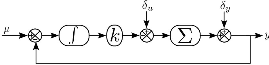
Figure S7: Integral feedback loop.
