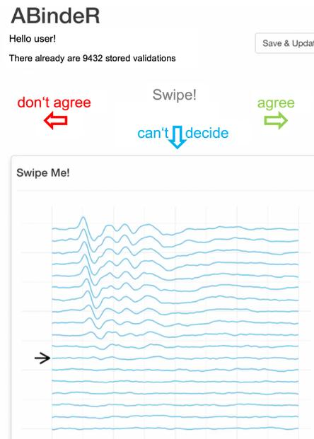
**Fig. 1: ABR threshold validation app used on standard tablet computers.** Users are presented a randomly selected ABR measurement along with the original human-assigned threshold, visually indicated by an arrow. Users can enter their evaluation by swiping left: “don’t agree”, right: “agree”, down: “can’t decide”. No mouse or stimulus information is provided in order to allow unbiased evaluation.
