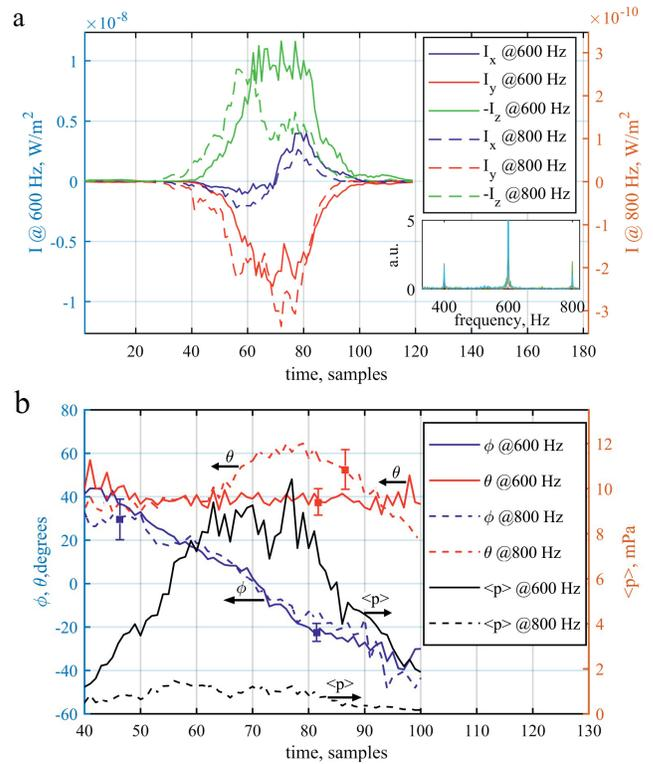
Figure 4. The temporal evolution of the orthogonal components of the acoustic intensity vector (a) and the directional angles together with the average acoustic pressure (b) obtained at the frequencies 600 Hz and 800 Hz during the acoustic source movement. The inset at the upper figure shows the Fourier-spectrum of the received acoustic signal.
