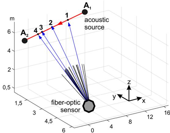
Figure 5. Experimentally obtained bearing vectors (black) and their continuations (blue) to the acoustic source and moving along the linear trajectory (red). Points 1, 2, 3 and 4 correspond to time moments of 40th, 60th, 70th and 75th samples, respectively.
