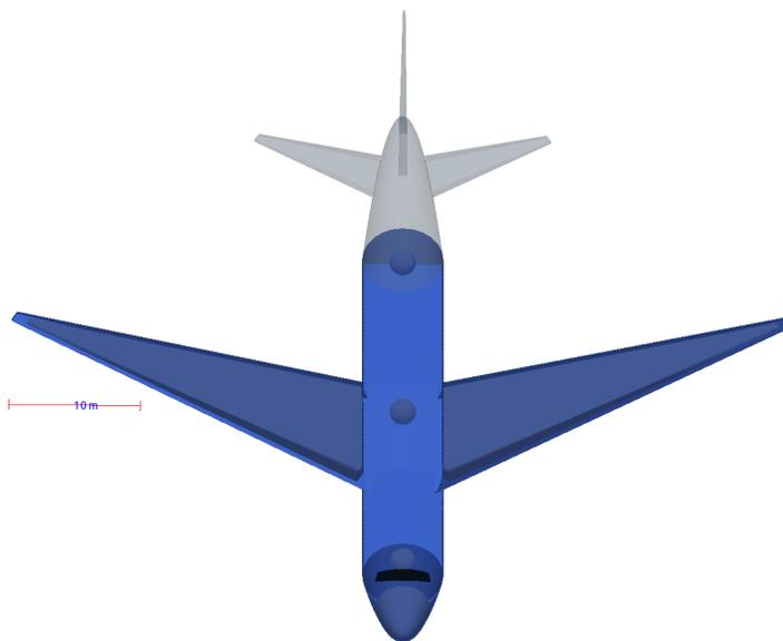
Figure 3: Mass model structure of the aircraft used in the simulation with three sampling dummy spheres placed at different sections inside the fuselage.
