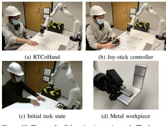
Figure 10: Photos of collaborative inspection task. The human users can interact with the cobot using either (a) RTCoHand framework or (b) joy-stick controller. Initially, the metal workpiece (d) is placed in a mold marked with black and yellow tape as shown in (c). Users need to first lift the workpiece out
