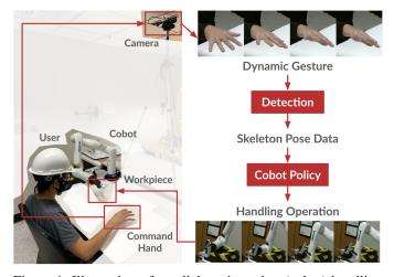
Figure 1: Illustration of a collaborative robot (cobot) handling task. Users control the workpiece handling operations using only dynamic gestures as commands. The dynamic gestures are first captured by multi-view cameras and then processed using skeleton detection toolbox. Then, a cobot policy maps user commands to handling operations, which are finally executed by the cobot in real time.
