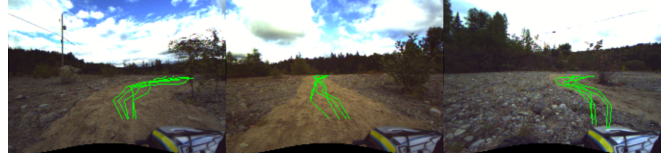
Fig. 8: High-scoring action rollouts moving towards smooth terrain output by the trajectory-attention planner when invoked on sample image inputs.
