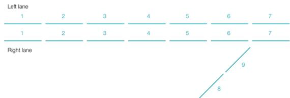
**Fig. 10:** Discretizing the double-lane scenario from Figure 5 into CTM cells.
