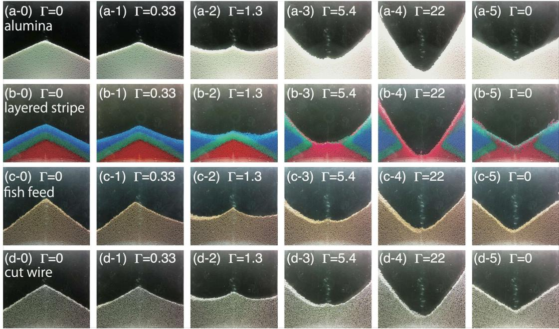
Figure 3: Raw image data of the granular pile deformation. Granular piles consisting of (a) alumina beads, (b) colored glass beads (with layered-stripe structure), (c) fish-feed particles, and (d) cut-wire particles are shown. The left column shows the initial shape, and the right column displays the final shape. Corresponding  $\Gamma$  conditions are denoted in each panel.
