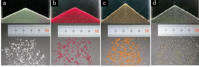
Figure 2: Pictures of grains used in this study, (a) alumina beads, (b) colored glass bead, (c) fish-feed particles, and (d) cut-wire particles are shown. The upper and lower rows show the piles and grains, respectively.
