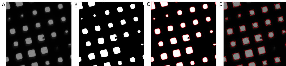
**Figure 2. Example of the square localization procedure.** A. Original input image. B. Mask recovered after segmenting pixels. C. Finding convex polygons around the separate regions in the mask. D. Aligned minimum bounding rectangles around the polygons, used for crops of the images.
