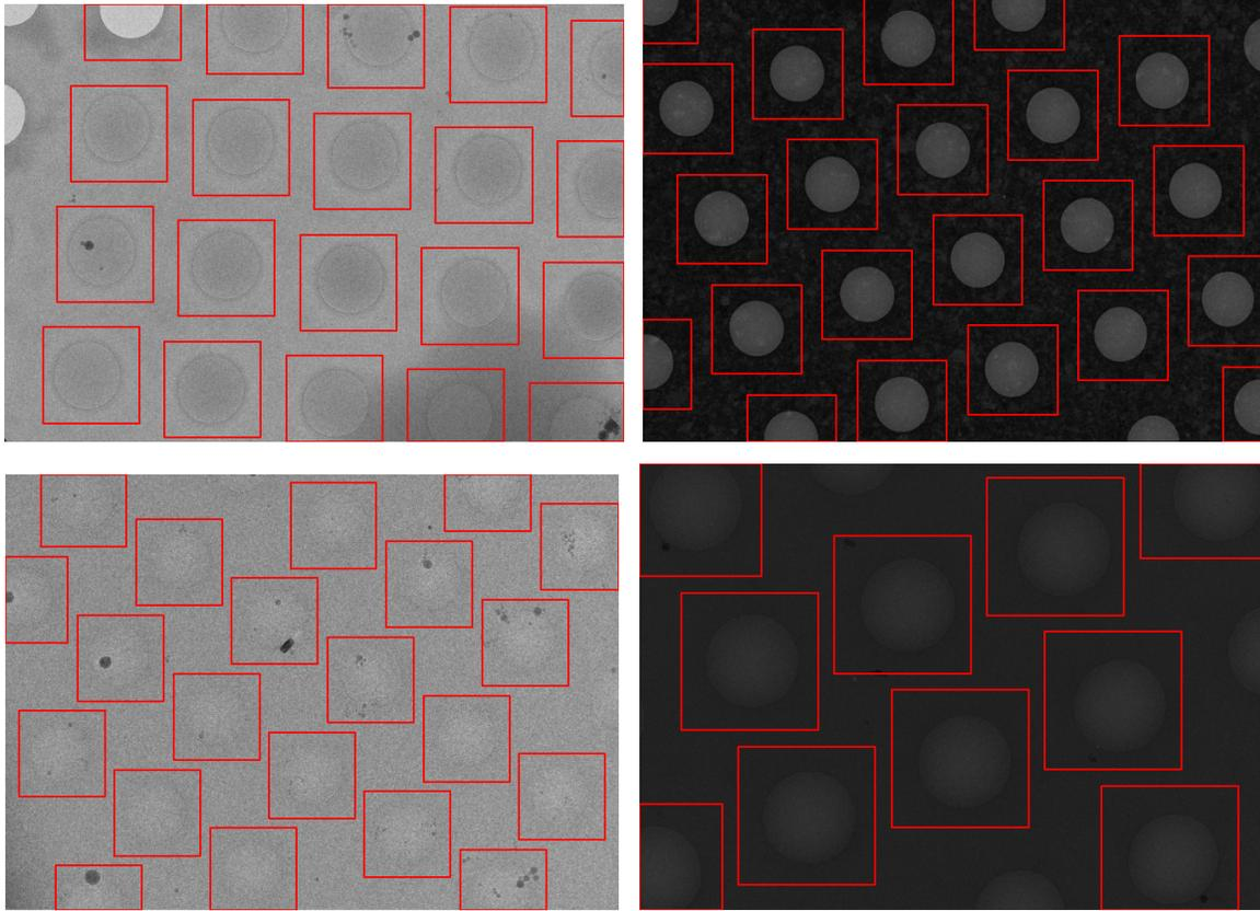
**Figure 9. Examples of hole localization using the U-Net + Lattice Fitting.** The model successfully detects all holes across a wide range of hole sizes, brightness, and contrast conditions, from easily visible gold grids (top right) to very low contrast carbon grids that are difficult to see even for humans (bottom left).
