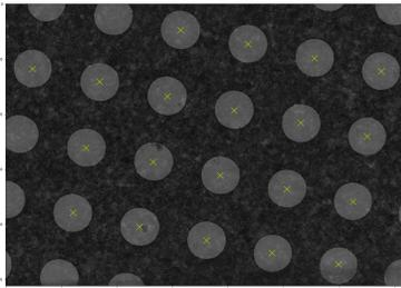
**Figure 3. Example medium-mag image** Selection locations are marked in yellow. The input to the U-Net is the image without any marking for the selection locations, while the output is a map with a 1 at each pixel where a selection occurred and 0 elsewhere.
