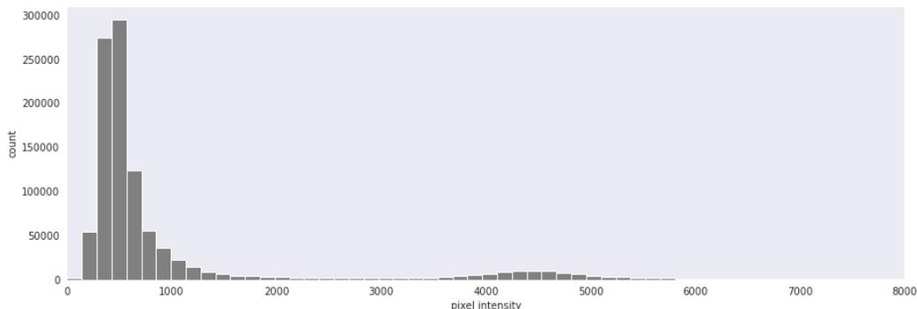
**Appendix Figure S1. Histogram of pixel intensities for an example low-mag image.** The pixel intensities from the squares and the grid bars decompose into two separate distributions with little overlap, thereby allowing a mixture model to separate pixels into two classes.
