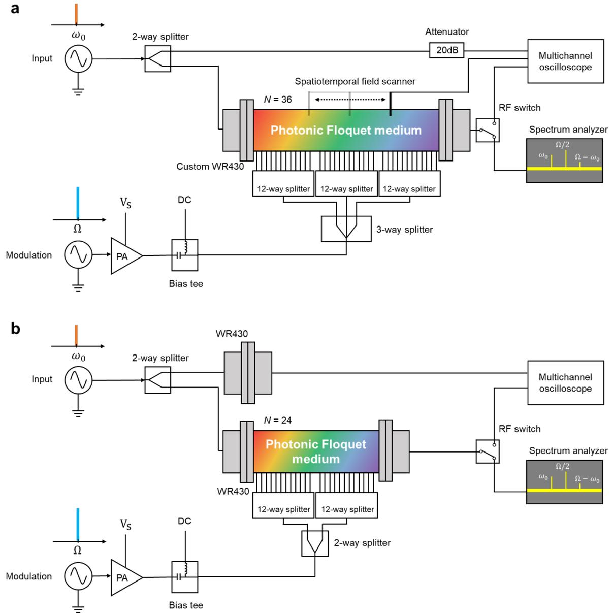
**Supplementary Figure S8. Schematics of the experimental setups.** (a) Schematic diagrams of the spatiotemporal field probing measurement setup and (b) phase retardation measurement setup. Here, the acronyms are as follows. PA: power amplifier;  $V_S$ : supply voltage;  $N$ : number of unit cells; DC: direct current; WR430: rectangular waveguide with opening dimensions of  $4.30 \times 2.15$  inches.
