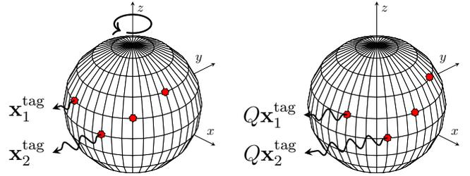
Fig. 2: Rotation of the object about the  $z$ -axis. When the object rotates, the tags rotate along with it. The new positions of the tags produce a different received signal. While the tags are equidistant from the point of rotation in the figure, this does not have to be the case.
