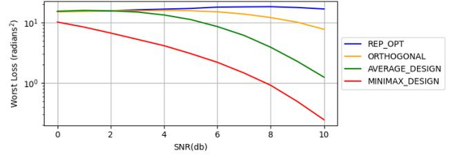
Fig. 9: The worst-case error versus SNR for the tag array in Figure 6. At an SNR value of 10dB, the designed code for the worst-case error is nearly 100× more accurate than the orthogonal code.
