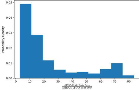
Fig. 8: Probability density histogram of the average error ratios when using the orthogonal code and the designed code at an SNR of 10dB.
