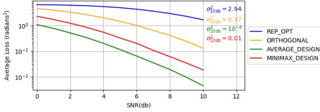
Fig. 7: The average squared error versus SNR for the tag array in Figure 6. At an SNR value of 10dB, the designed code for the average error is nearly 70× more accurate than the channel-agnostic orthogonal code.
