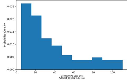
Fig. 10: Probability density histogram of the worst error ratios when using the orthogonal code and the designed code at an SNR of 10dB.
