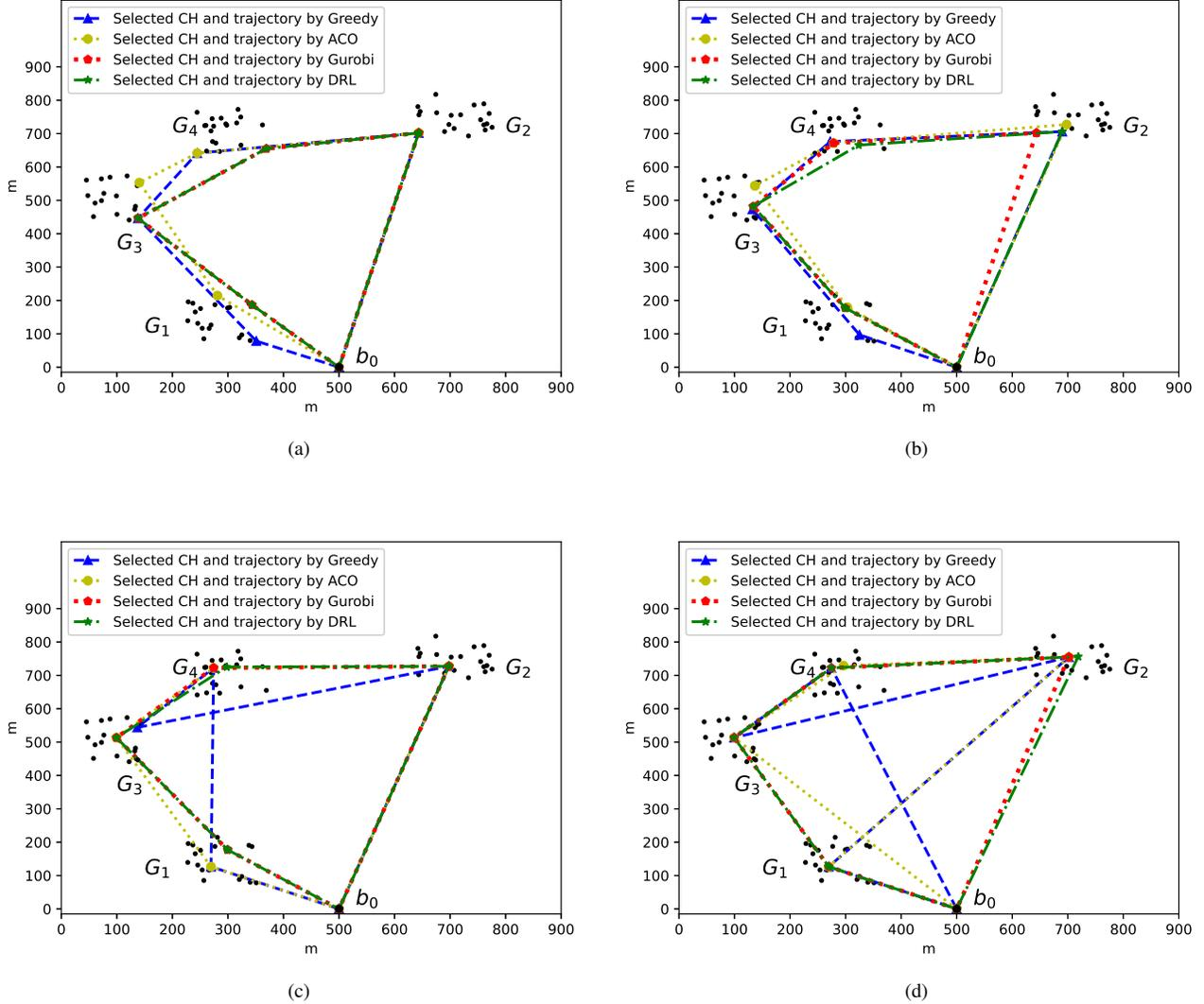
Fig. 4. Trajectory comparison of DRL, greedy algorithm, ACO, and Gurobi for different values of  $\omega$ . (a)  $\omega = 0$ . (b)  $\omega = 0.3$ . (c)  $\omega = 0.6$ . (d)  $\omega = 0.9$ .
