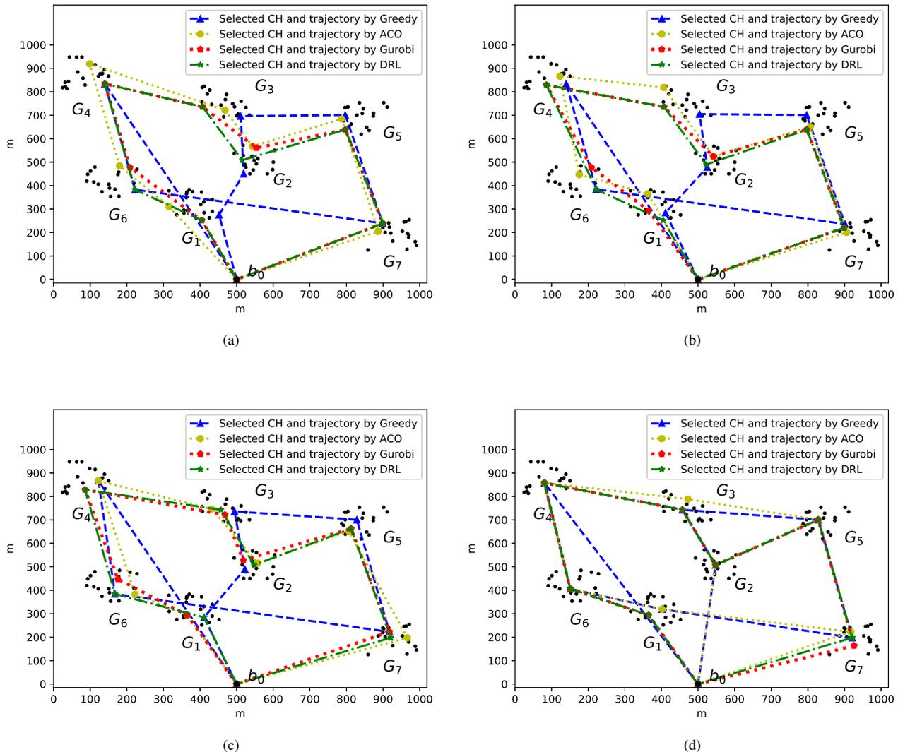
Fig. 6. Trajectory comparison of DRL, greedy algorithm, ACO, and Gurobi for different values of  $\omega$ . (a)  $\omega = 0.1$ . (b)  $\omega = 0.3$ . (c)  $\omega = 0.5$ . (d)  $\omega = 0.8$ .
