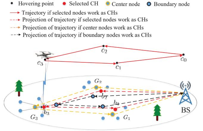
Fig. 1. System model of an UAV-aided cluster-based IoT network.
