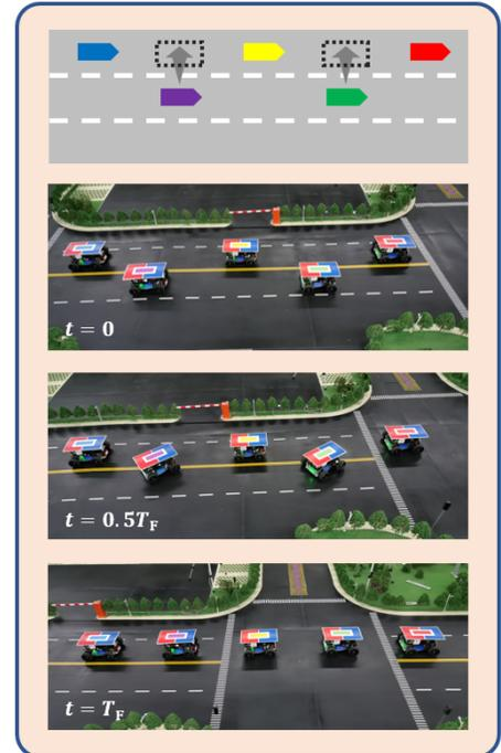
(c) Formation switching from two-lane structure to one-lane structure
