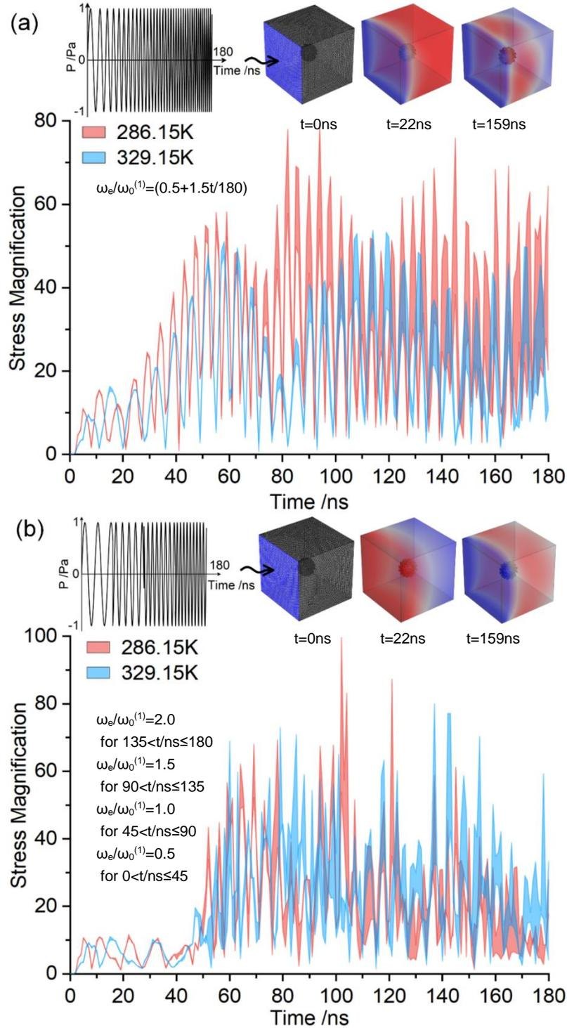
**Fig. 4. Stress magnification around the root of swung spike excited by ultrasound wave of frequency  $\omega_e$  that change (a) continuously and (b) step-wisely with time, along with acoustic pressure, stress field and the initial wave profiles of the ultrasonic waves for the cases of temperature  $T=286.15K$ .**
