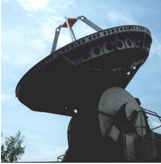
Fig. 2. Antenna with plate near Moscow, radar target used in [6] with ERS SAR.
