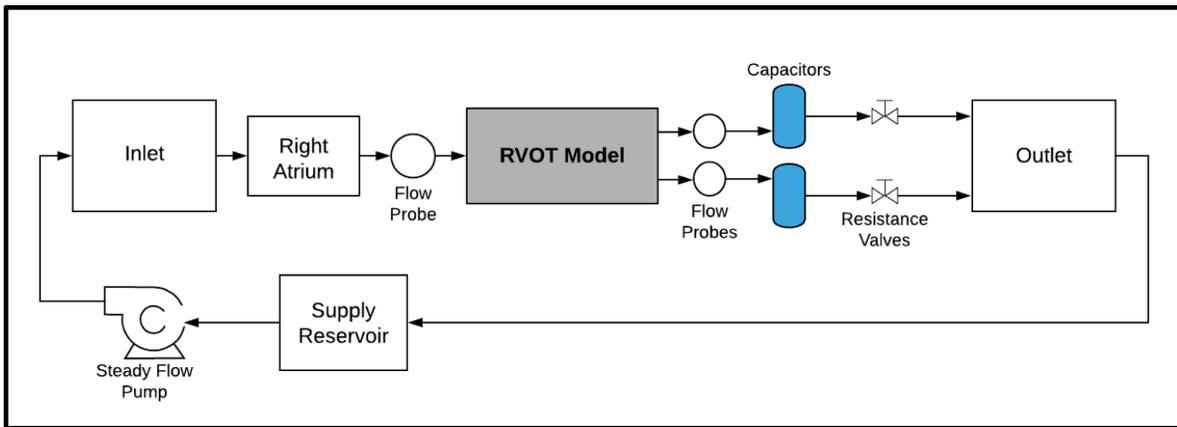
Figure 3: Schematic of the experimental flow loop.
