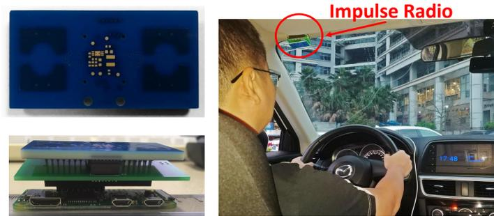
Fig. 19. COTS impulse radio used in V<sup>2</sup>iFi and radio setup inside the vehicle.
