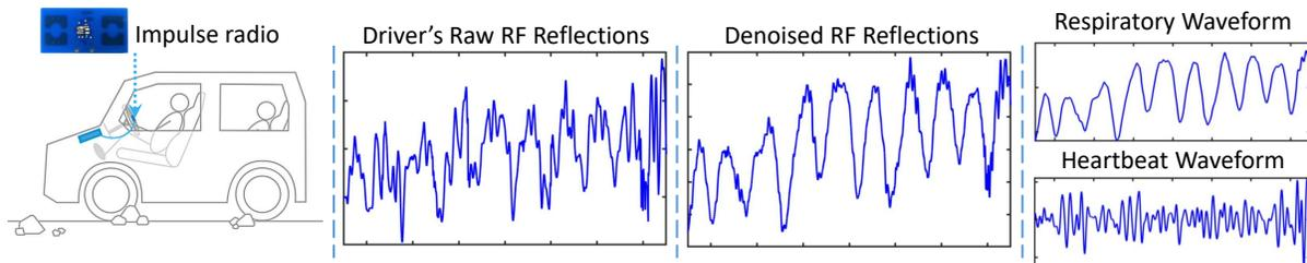
Fig. 2. A vital signs monitoring scenario of driving vehicle. The driver's RF reflections always contains his or her vital signs with noise introduced by vehicle's vibrations. V<sup>2</sup>iFi separates such vibrations to reconstruct signals of vital signs.
