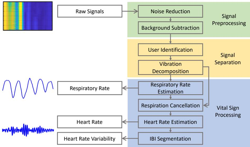
Fig. 3. Software system design of V<sup>2</sup>iFi.
