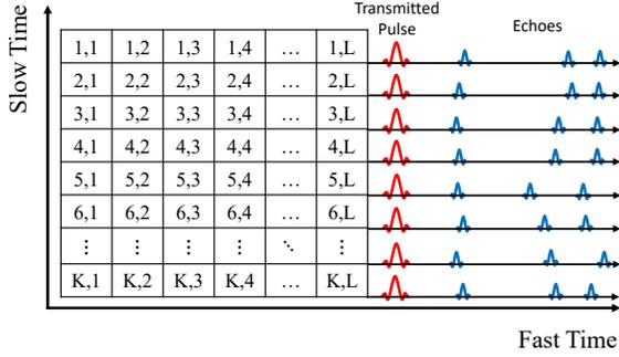
Fig. 7. The matrix of received baseband signals.
