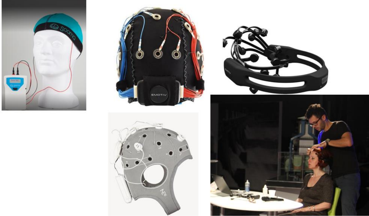
Figure 3. Illustration of possible EEG recordings, standard and portable (on this picture there are two members of our team, the author of this paper included, not the patients. The photo was made during our public demonstration during SUTRA festival of science in Republic Serbia in 2019, https://www.youtube.com/watch?v=pHAFfliOTo&ab_channel=Milena%C4%8Cuki%C4%87 ).
