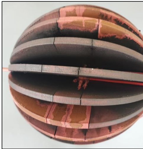
Figure 5.16: Partially coated fin sphere.
