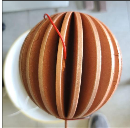
Figure 5.17: Successfully electroplated fin sphere ground.
