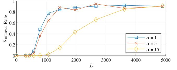
**Fig. 3.** Success rates of Algorithm 1 to recover the block structure  $\mathcal{B}$  as a function of the number of snapshots  $L$  and different ratios  $\alpha = \frac{M}{pN}$ . Herein,  $N = 1000$ ,  $M = 400$  and  $d = 20$ . Results are averaged over 200 trials.
