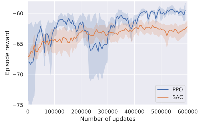
Fig. 10. Performances with respect to the number of updates. The training with off-policy SAC is more stable, but eventually only learns the locally optimal policies. While, the training with on-policy PPO can learn the policies with better performance.
