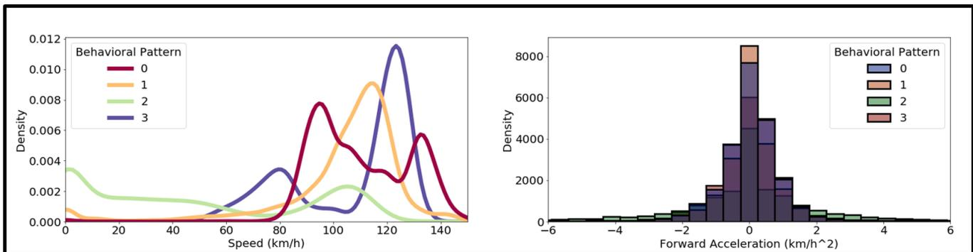
Fig. 10. The distribution of forward acceleration and speed across different patterns retrieved unsupervised from 12 participants. Note that because we retrieved accelerometer data from the low resolution speed, the distributions are less smooth as compared to case study I. Thus, we are visualizing the differences across driving patterns with a histogram instead of a kernel density estimation (KDE).
