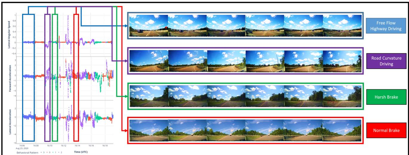
Fig. 5. Samples of the detected driving patterns. Patterns 0 and 1 are associated with normal and harsh braking behavior, while pattern 2 is associated to curve driving behavior, and pattern 3 is related to highway free flow driving behavior.
