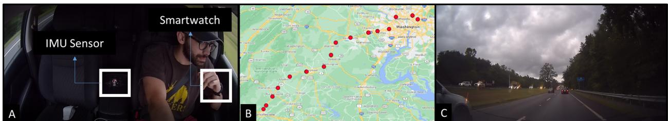
Fig. 2. An overview of the case study dataset. The vehicle is equipped with a camera, smart watch, and an IMU sensor (A, and C). The data is collected from a 120 mile driving scenario between cities of Charlottesville and Washington DC, with a duration of 2 hour and 10 minutes (B).
