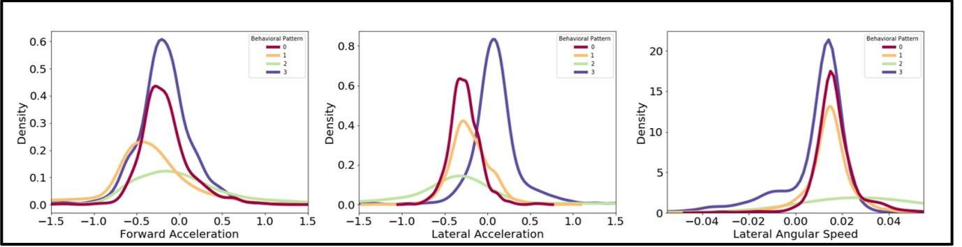
Fig. 4. Distribution of different kinematic sensor readings within different driving patterns. Note that differences across patterns in the kinematic sensor distributions, for instance, pattern 3 has a more positive lateral acceleration than the other 3 patterns. Also note that for some patterns the difference is only visible through one sensor such as the comparison between patterns 0 and 3 lateral acceleration.
