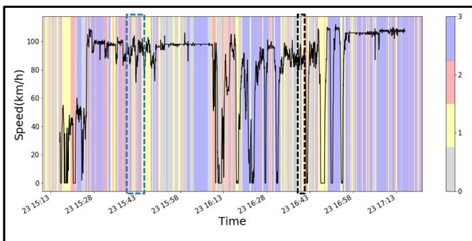
Fig. 6. The change in driving patterns throughout the different segments of driving. Each segment is associated with one of the four driving patterns as described previously. Note that when speed changes more sporadically, the behavior also changes more often (e.g., blue dashed box). Also, the black dashed box shows a sequence of sample behavior starting from free flow highway driving, switching to road curvature driving, and finishing with a harsh brake.
