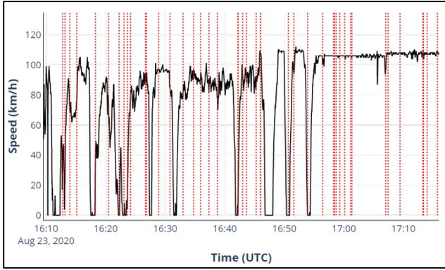
Fig. 3. Different segments of driving detected by the BCP applied on the kinematics data shown with dashed vertical lines.
