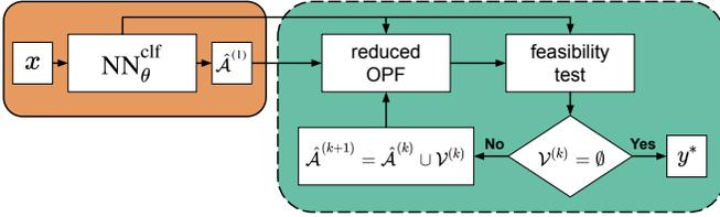
Fig. 3. Flowchart of the iterative feasibility test method (green panel) combined with a NN classifier (orange panel).  $\hat{\mathcal{A}}^{(k)}$  and  $\mathcal{V}^{(k)}$  are the sets of predicted active and violated inequality constraints at the  $k$ -th step of the iterative feasibility test, respectively. For clarity, default arguments of the OPF operator are omitted.
