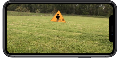
(b) FirstResponse-AR interface allowing on scene rescue team members to visualize geolocated markers using AR Glasses and AR mobile apps
