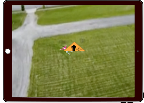
(b) The system persists the geolocation of the POI (Injured Person) identified in the aerial video stream of the UAV-1. Therefore, Flying-AR uses it to augment the video stream of UAV-2 in the same mission with an appropriate marker when its camera looks towards the POI's geolocation.
