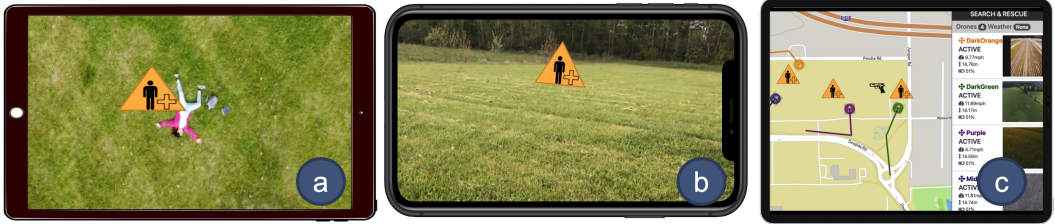
Fig. 1. RescueAR utilizes location-based augmented reality technology to facilitate the exchange of information among rescue team members during a UAV-driven emergency response. (a) Flying-AR : Allows remote monitoring teams to mark the injured person in the aerial video stream from a UAV. (b) FirstResponse-AR : Allows on-scene first response team members to visualize the location of the identified injured victim in (a) using AR glasses or mobile devices. (c) Mission-Control : Allows mission planning team to visualize the spatial summary of the mission including the location of UAVs, their aerial video stream, and points of interest identified via (a)
