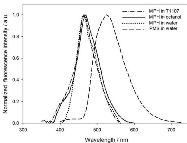
**Fig. 2.** Normalized emission spectra of PMS in water, and methyl-phenazine (MPH) in n-octanol, lipophilic micelles (T1107) and water.
