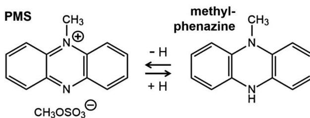
**Fig. 1.** Chemical structures of phenazine methosulfate in its oxidized cationic form (PMS), and the reduced derivative, methyl-phenazine. The incorporation of a hydrogen at the N atom of the central ring in PMS leads to a lower delocalization of the electrons, resulting in a color loss of methyl-phenazine.
