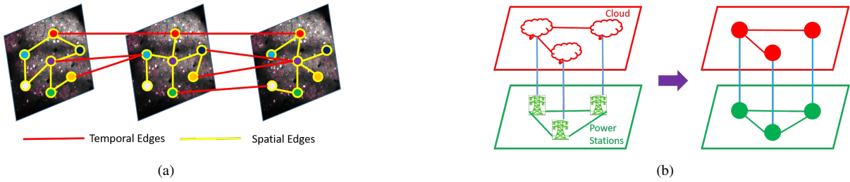
Fig. 1. Multilayer Graphs and Applications: (a) Video: each layer represents one frame of the video and the edges capture the spatial-temporal relationships; (b) Cyber-Physical System (CPS): each layer represents one component in CPS and the edges capture the physical connections.
