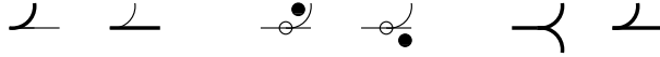
Figure 4 The switches used in the railway circuit of the model. To left, the fixed switch, in the middle, the flip-flop switch, to right the memory switch. In the flip-flop switch, the bullet indicates which track has to be taken.
