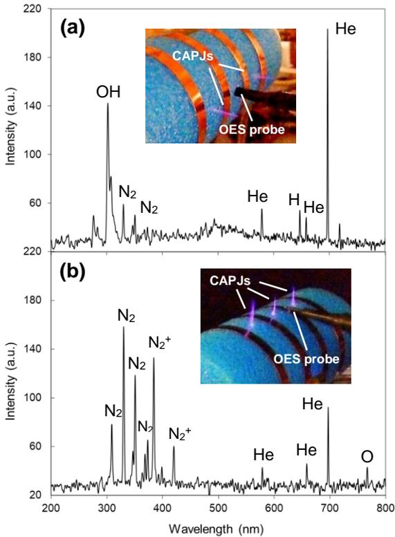
FIG. 4. Optical emission spectra from the He CAPJs measured (a) in the active DBD zone and (b) in the afterglow zone. The optically active plasma species are identified. Total He rate was 4 slm. Insets: images of the OES probe position with respect to the CAPJs.
