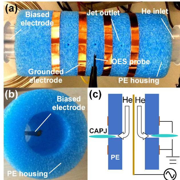
FIG. 1. (a) Image of the cylindrical plasma source showing the different parts. (b) Detail of the DBD active zone, comprised between the biased (core) electrode and the flexible PE spacer. (c) Schematic cross section of the plasma source. The working principle of the radial CAPJ generation in the afterglow zone is indicated.
