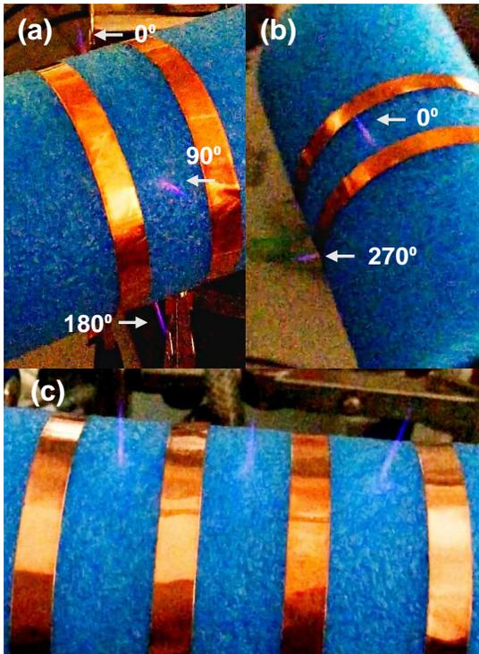
FIG. 2. Images of the He CAPJs striking in the (a,b) brush mode (8 slm He) and (c) the comb mode (6 slm He). The jet positions at  $0^\circ$ ,  $90^\circ$ ,  $180^\circ$  and  $270^\circ$  in (a) and (b) are indicated with arrows. Two grounded electrodes were used in the brush mode, whereas four grounded electrodes were necessary to obtain CAPJs in the comb mode.
