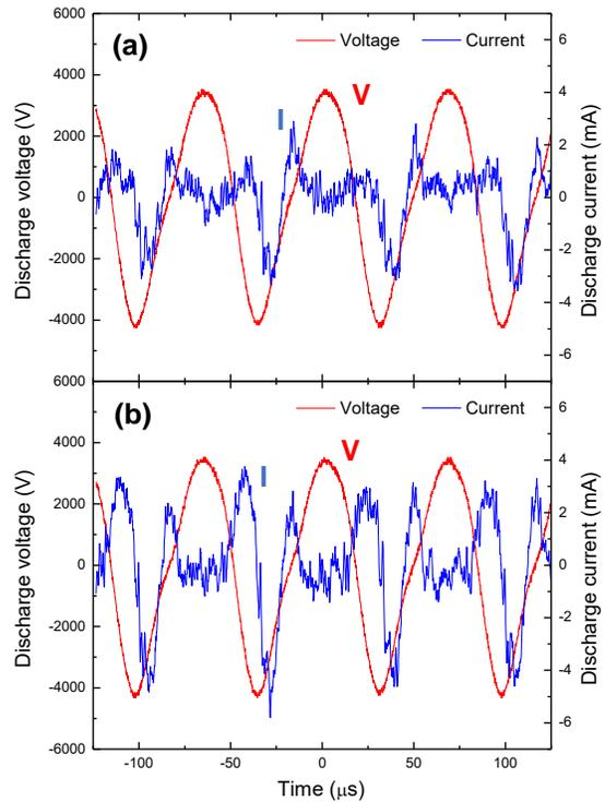
FIG. 3. Current (blue) and voltage (red) waveforms corresponding to He CAPJs ignited in (a) brush mode at 8 slm and (b) comb mode at 6 slm.
