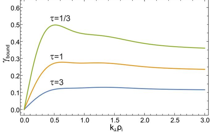
FIG. 1: Upper bound (11) on the growth rate (in arbitrary units) of gyrokinetic instabilities for  $k_{\psi} = 0$  and three different values of  $\tau = T_i/T_e$  in a plasma with adiabatic electrons as a function of the smallest value of  $k_{\perp} \rho_i$  along the magnetic field.
