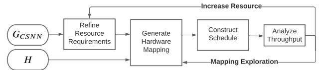
Fig. 6. Design space exploration to perform throughput-buffer size trade-off.
