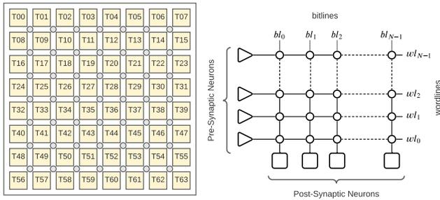
(a) A many-core neuromorphic hardware. (b) Analog crossbar-based PE.
