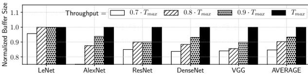
Fig. 11. Minimum buffer size for different throughput constraints.
