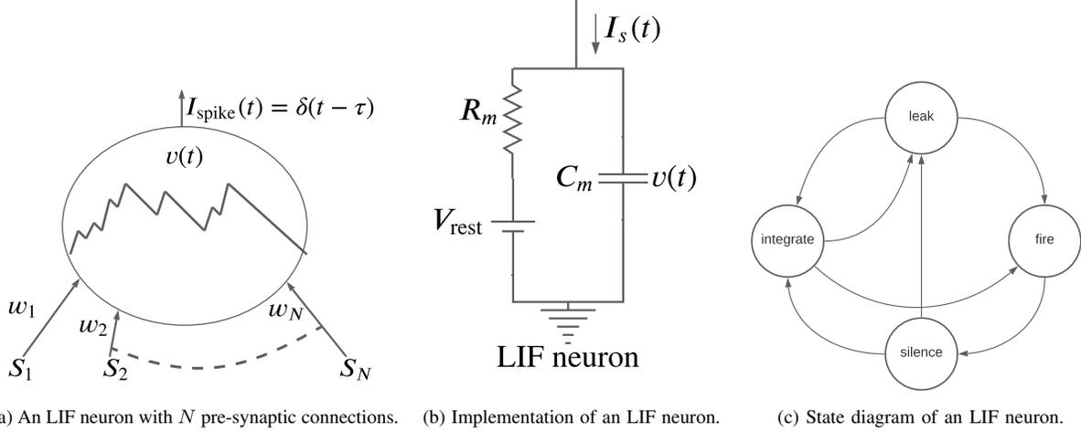
(a) An LIF neuron with  $N$  pre-synaptic connections. (b) Implementation of an LIF neuron. (c) State diagram of an LIF neuron.
