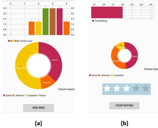
Fig. 6. App UI (a) App interface showing comfort levels at intervals and impact of speed, congestion and jerkiness over the comfort. (b) The overall rating unit of the app. (1 - Most Comfortable, 5 - Most Uncomfortable)
