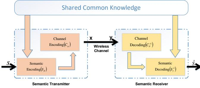
Fig. 1. The general framework of semantic communication system.
