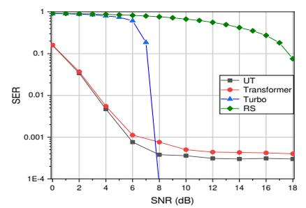
Fig. 5. SER score versus SNR in AWGN channel.
