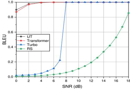
Fig. 3. BLEU score versus SNR in AWGN channel.
