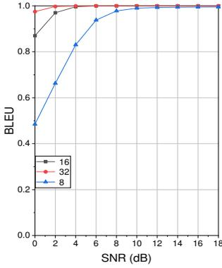
Fig. 6. BLEU versus the number of symbols used for in one word in semantic communication.
