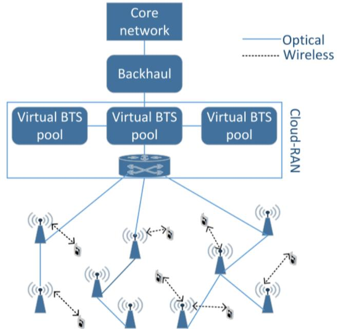
Fig. 3: The architecture of CRAN in 5G networks. CRANs combine baseband processing units of a group of base stations into a central server retaining radio front end at the cell sides.
