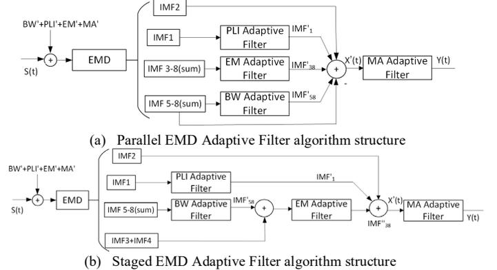
Fig. 4. Proposed Algorithm Structure to Denoise ECG Contaminated by BW+PLI+EM+MA Based on EMD and Adaptive Filter
