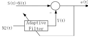
Fig. 1. Applied adaptive filter structure
