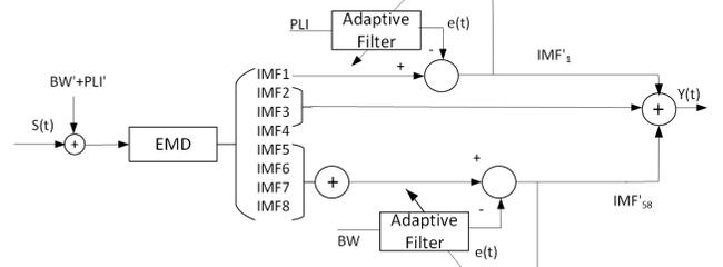
Fig. 3. Proposed algorithm structure to eliminate BW and PLI noise
