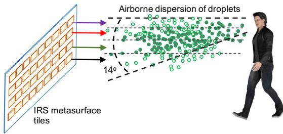
Fig. 3. The dispersion of droplets through the air can take between  $1 - 14^\circ$  in environments with no evaporation (after an initial expulsion of  $27.5^\circ$ ) [5].
