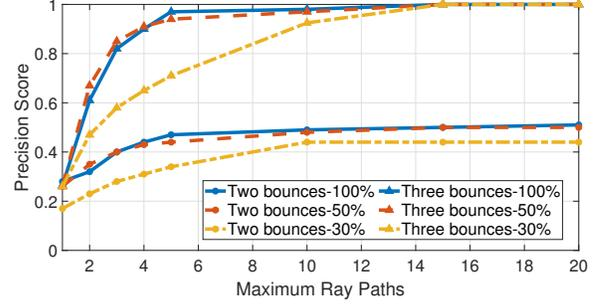
Fig. 5. Precision score versus maximum number of two-bounce or three-bounce ray paths per scanned grid. Results are presented for an IRS coverage of 100%, 50%, and 30%.
