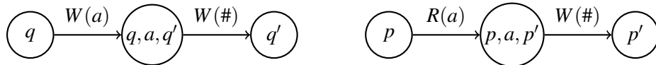
Figure 3: Simulation in \mathcal{P} of transitions q \xrightarrow{!a} q' and p \xrightarrow{?a} p' of \mathcal{R} .
