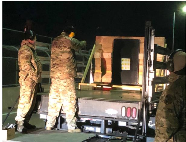
FIG. 11. Firing Position 1, showing the shooter and bullet trap, illustrating the source of the signals used for the test.
