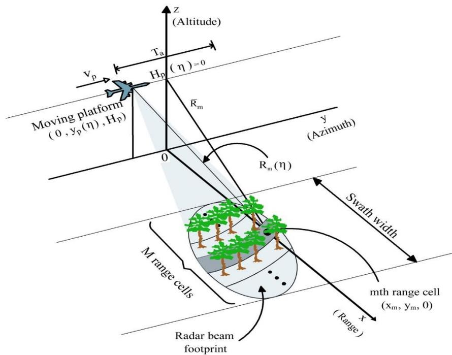
Fig. 1. Geometry of stripmap SAR FOPEN
