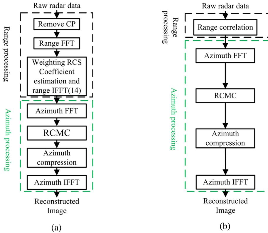
Fig. 2. Block diagram of SAR imaging processing. (a) CP-based OFDM SAR. (b) Random noise SAR
