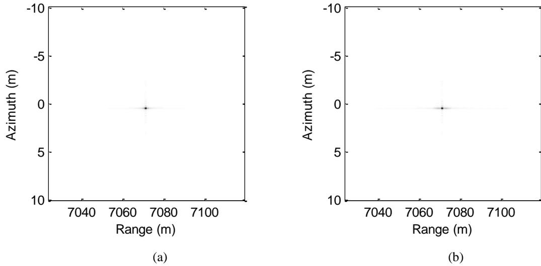
*Fig. 6. Single point target Imaging results of UWB SAR FOPEN. (a) CP-based OFDM SAR FOPEN, HH. (b) Random noise SAR FOPEN, HH.*
