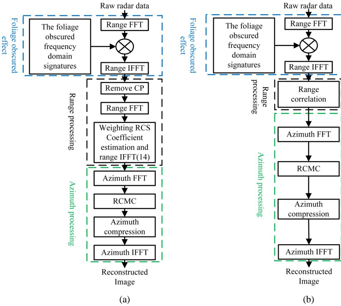
Fig. 4. Block diagram of UWB SAR imaging process for FOPEN. (a) CP-OFDM signal. (b) Random noise signal
