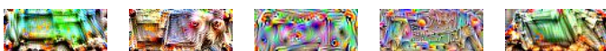
Fig. 16: Visualization of the 6% rectangular adversarial patch (36*88*3) on ImageNet. From left to right: ResNet-50, DenseNet-121, SqueezeNet, VGG16 and ResNet-152. Same for Fig. 17 and Fig. 18.
